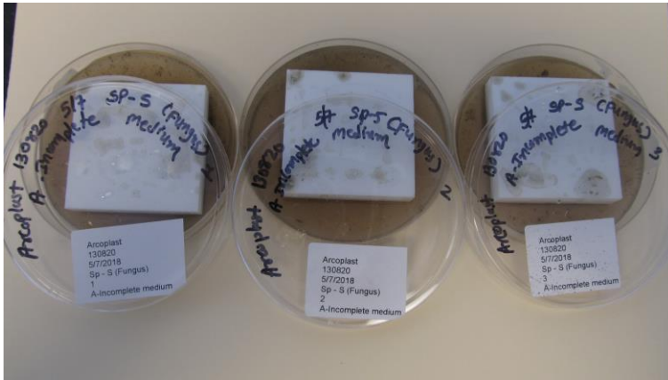
Figure 1: Method A- Fungal spore inoculated to the surface of test sample and Mineral salt agar © Accugen Labs
