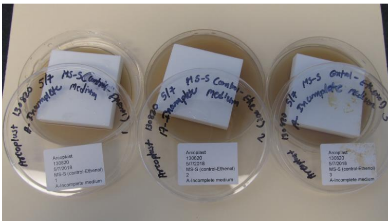
Figure 2: Method A- Microbiocidal solution added to the surface of test sample on Mineral salt Agar @Accugen Labs
