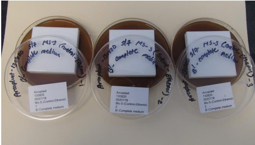
Figure 7: Method B' Microbiocidal solution added to the surface of Mineral salt Agar with glucose and test sample @Accugen
