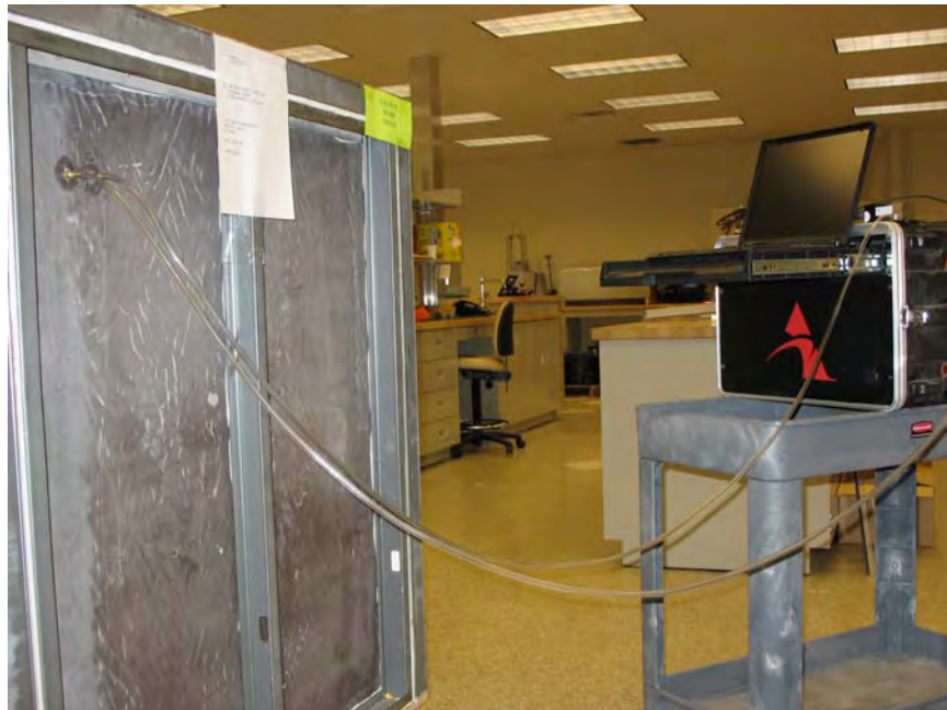
Photo No. 2 Connection of Module to Computerized Data Collector
