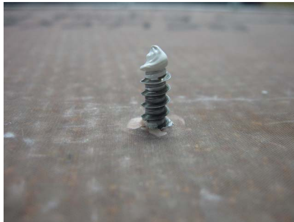
Panel 4 – Screw seen from non-gel side; screw head on gel side of panel holds a bracket
