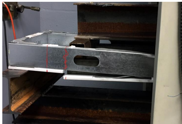
Figure 10: Sample #5,6 Typical Failure
