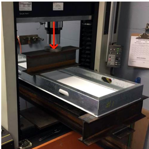
Figure 1: Sample #1,2 Test Set Up
