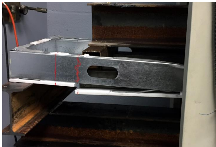
Figure 10: Sample #5,6 Typical Failure
