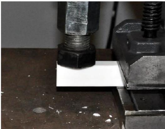
Figure 3a: photo of solid panel seismic shear test
